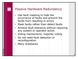
Passive Hardware Redundancy
