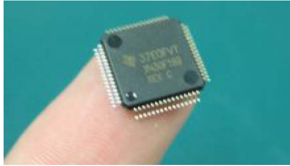
Figure 4-1. Microcontroller Texas Instruments MSP430F169.
