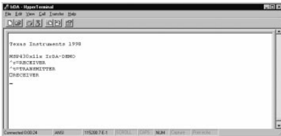
Figure 6. IrDA Initialization Acknowledgement – Receiver
