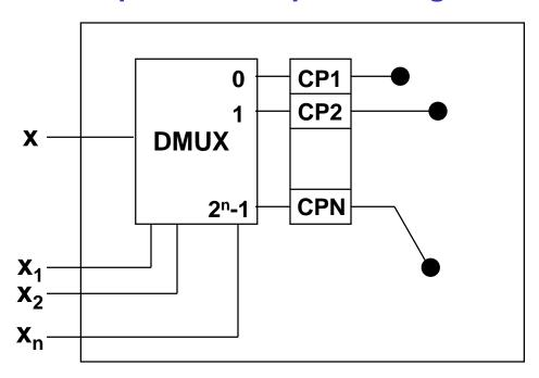
To reduce the number of input pins for controlling testpoints, demultiplexer and a latch register can be used.
