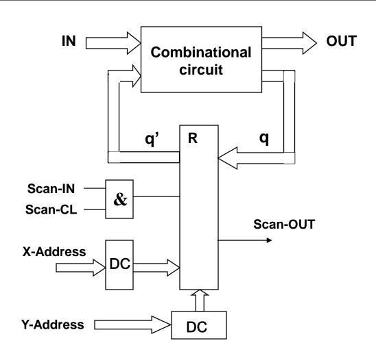
In random access scan each flip-flop in a logic network is selected individually by an address for control and observation of its state
