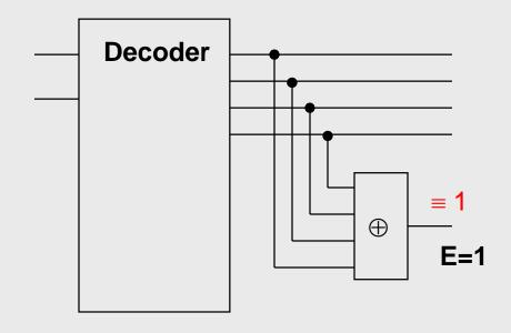
E = 1 if decoder is fault-free Fault ≡ 1 is not testable
