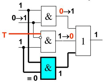
Redundant AND-gate Fault ≡ 0 not testable
