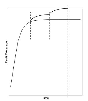
**Problem: low fault coverage** → long PR test
