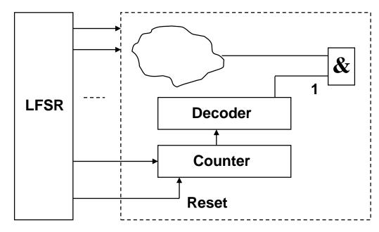
If Reset = 1 signal has probability 0,5 then counter will not work and 1 for AND gate may never be produced
