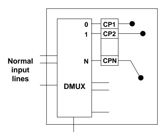
To reduce the number of input pins for controlling test points, time-sharing of working inputs can be introduced.
