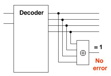
E = 1 if decoder is fault-free Fault ≡ 1 not testable
