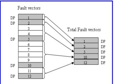
Diagnostic Points (DPs) – patterns that detect new faults Further minimization of DPs – as a tradeoff with diagnostic resolution
